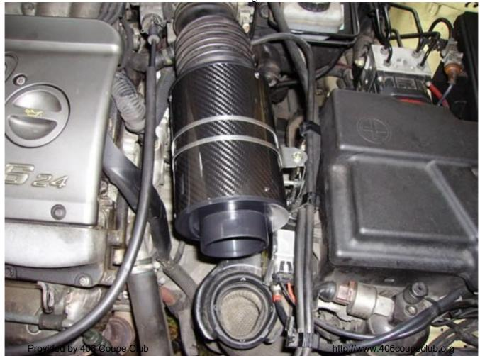
You'll see it's only an inch, but it gives you that little extra room for the flexi pipe to neatly curve onto the inlet part of the filter, remember (if you need to) use one of the reducer rings to fit it into the main air pipe. After moving it back:
