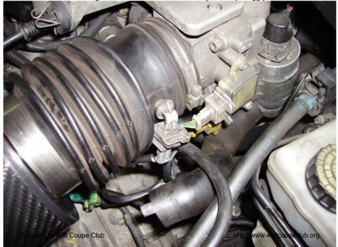
Next up was to fit the ICV breather filter to the original breather pipe, this was simple. The original pipe is 1" / 25mm.
