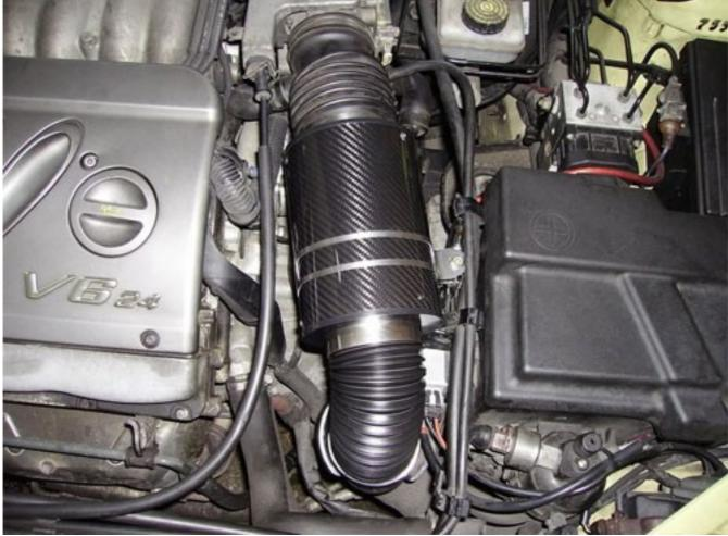
It's here that you will now need to trim an appropriate length of the new air feed pipe, measure it up so that it fits over the filter, has a nice bend to it and sits in the coupes air intake. Trim it accordingly using the wire snips. Next up was to drill a small hole for the IAT sensor to be relocated. Can't remember the exact size as I used funny imperial
