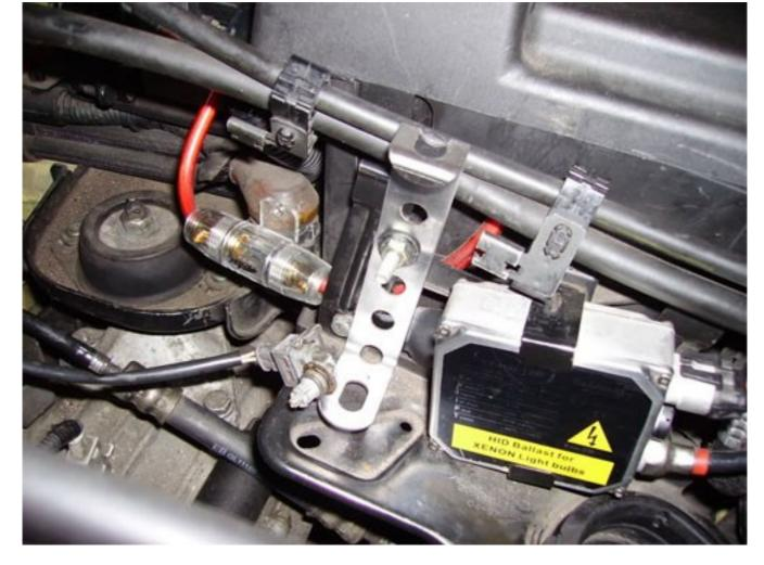
Now with that in place, we start to build the kit up. Carefully (without scratching the body) bring the body band up level with the top of the bracket, just hand tighten the nut & bolt. This is where the second pair of hands comes in, get someone to push the filter body back a bit to give you a bit more room at the front, whilst doing this tighten the but & bolt. Before moving it back:
