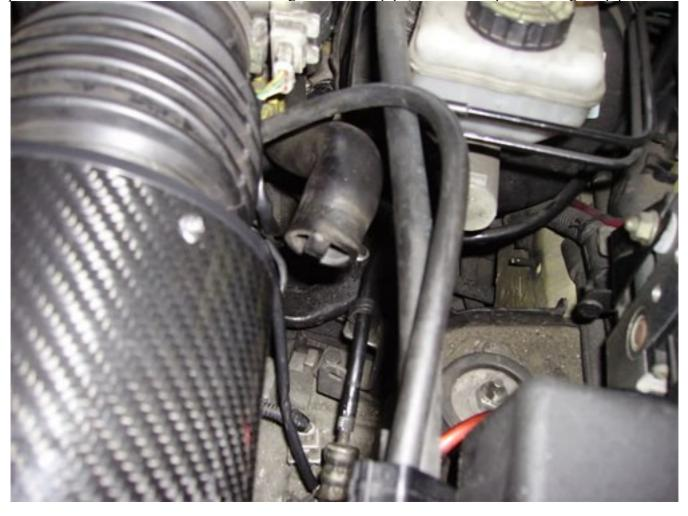
This is where the 1" joiner comes in as per the 2nd picture above. You can use a smaller one I suppose, but in my eyes, that pipe is 1" for a reason. Tighten the jubilee clip up that came with your small filter, this will secure the hose joiner to the small filter, then using the extra jubilee clip you got yourself, slide that over the breather pipe and tighten that over the other end of the pipe joiner / mender.
